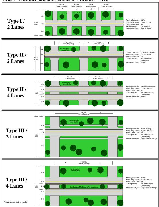
FIGURE 1: CONCEPTUAL SCHEMATICS OF ROADWAY TYPES
