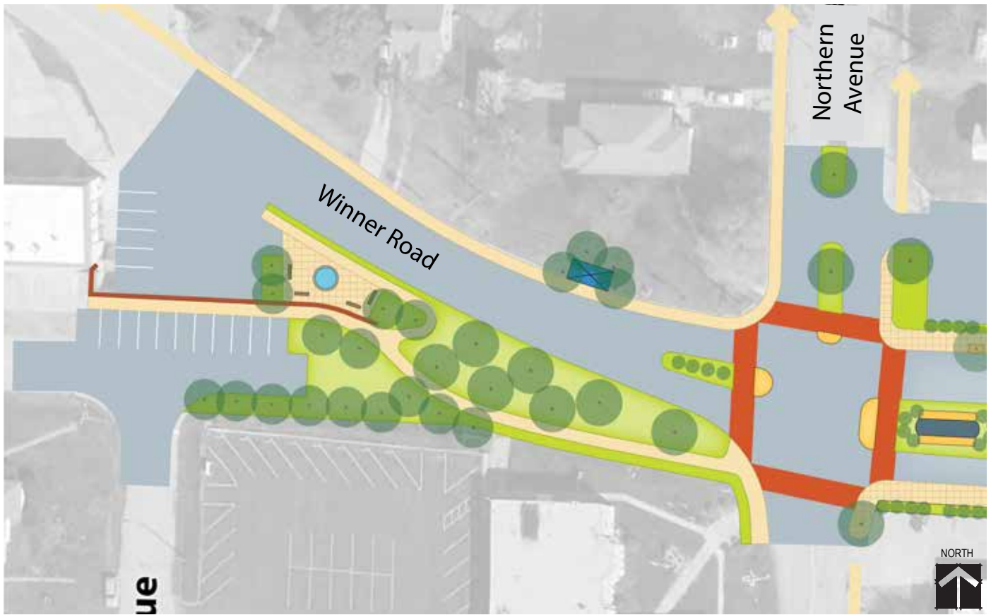
Figure 21 | Option One Winner Road and Northern Avenue intersection design, depicting the closing of 18th Street access.
