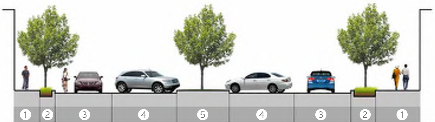
Proposed Design Section | 1. Sidewalk 2. Amenity zone 3. Shared-use lane 4. 45 degree angle parking 5. Green median
