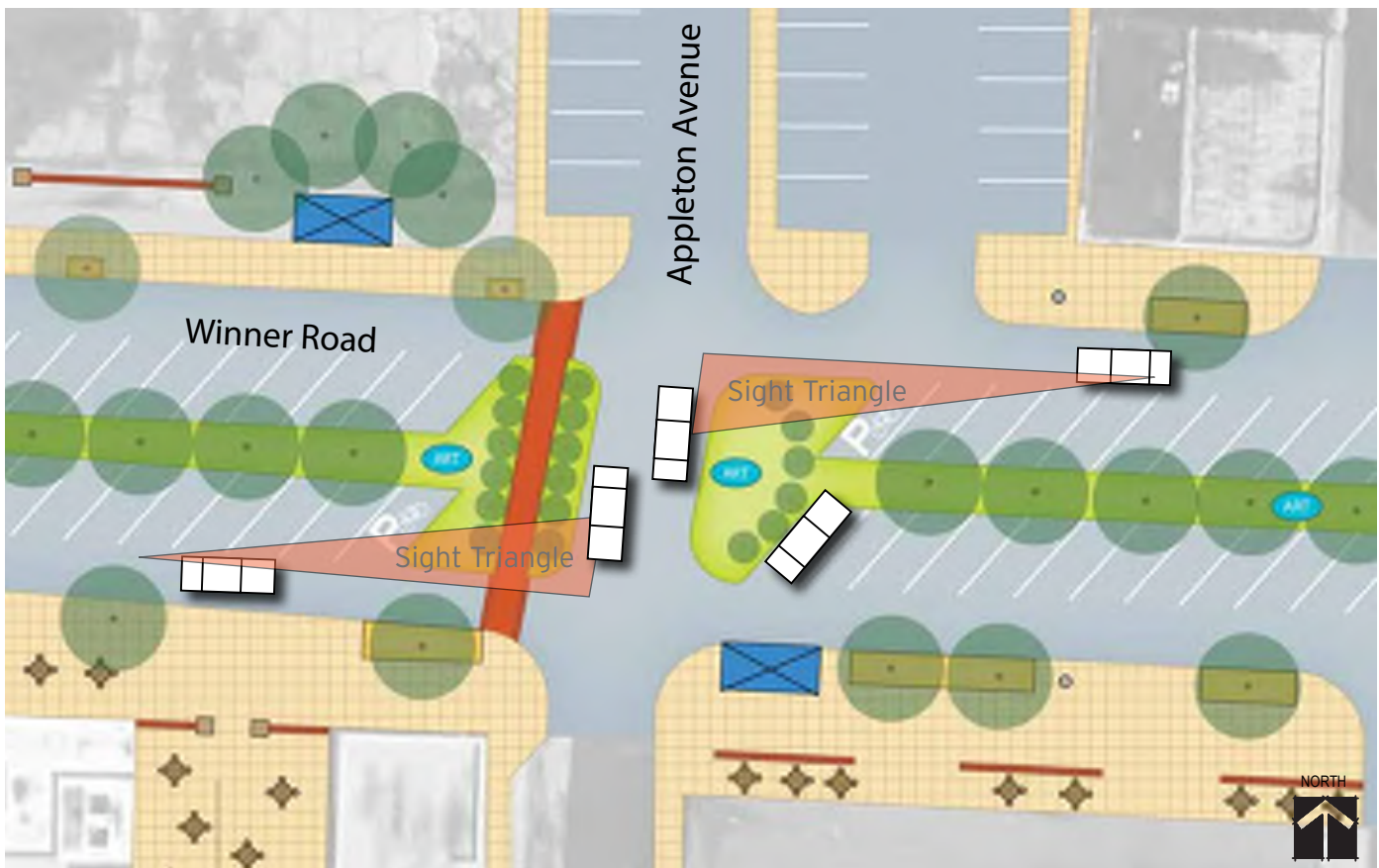
Figure 20 | Plan view of Appleton Avenue and Winner Road center turn sight triangles
